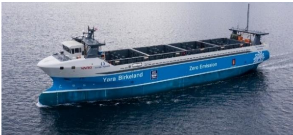
Yara Birkeland is the world's first fully electric and autonomous container vessel with zero emissions. Image © Kongsberg Maritime AS, 2024
