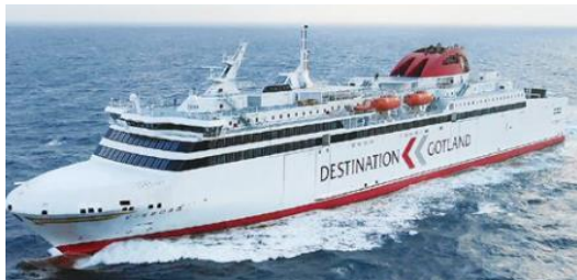
Ro-Ro passenger vessel powered by LNG-fuel oil dual-fuel engine. (Source: CSSC)
