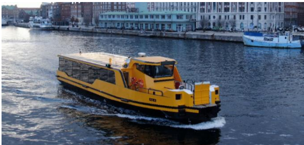
Fully electric passenger ferry in Rotterdam. (source: Damen Shipyard and Purus)
