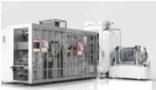
Coating, rolling and slitting integrated machine
